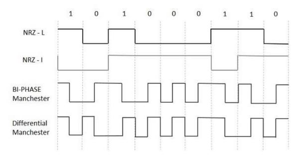
It is required that information must be encoded into signals before it can be transported across communication media. In more precise words we may say that the waveform pattern of voltage or current used to represent the 1s and 0s of a digital signal on a transmission link is called digital to digital line encoding. There are different encoding schemes available:
